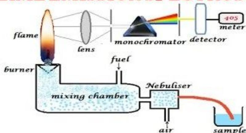
Volatilization of molecules in a flame produces free atoms and then excites them to higher energy levels. The characteristic emission spectrum of the element is produced when the excited atoms return to their ground state. **This is the principle of emission flame photometry.**
