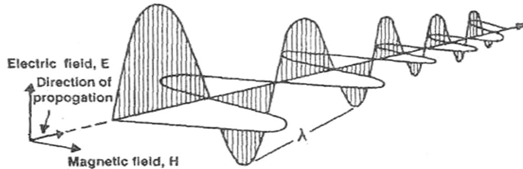
A beam of light from a bulb consists of many randomly oriented plane polarized components being propagated in the same direction. The distance along the direction of propagation for one complete cycle is known as **wavelength [ $\lambda$ ]**. Wavelength may be measured in centimeters (cm), micrometers ( $\mu\text{m}$ ), nanometers (nm) or angstrom units ( $\text{A}^\circ$ ).
