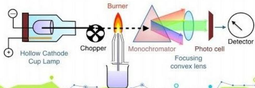
**Principle of Atomic absorption spectrophotometry**, to measures the absorption of a beam of mono-chromatic light by atoms in a flame.
